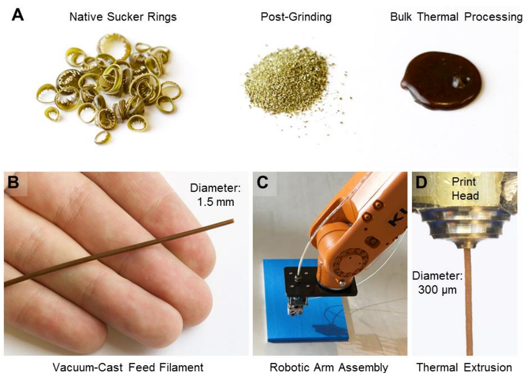
Figure 2.5 Thermal processing processes and extrusion of filaments from native SRT. (A) Native SRT were grounded into powder form, then mixed with plasticizing agents (50% SRT, 25% water and 25% glycerol by weight) and heated to 150 °C. (B) A 1.5 mm diameter feed filament was vacuum formed from the molten SRT mixture, which could then be (D) thermally extruded into a 300 μm diameter filament through a fused filament fabrication print head attached to a robotic arm (C). Figure reproduced from Ref. 10.
