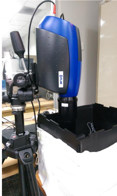
Figure A1-3: FLIR ® MWIR SC5000 thermal camera focused on black painted Gorilla Glass surface inside the black painted enclosure to minimize surrounding thermal irradiation reflection.
