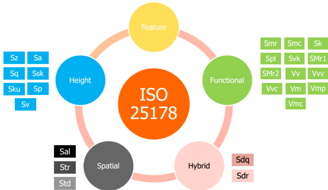
Figure 2-12. The surface texture parameters according to ISO 25178.
