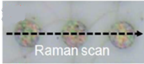
Figure 5.13: Schematic of high resolution Raman scanning along a TSV row prior to metallization.
