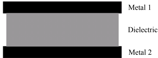
Figure 2.20: Capacitor formed by two metal lines and a dielectric layer in between.
