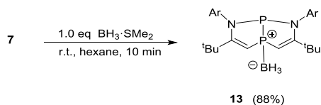
Scheme 4.8. Reaction of 7 with \text{BH}_3 .
