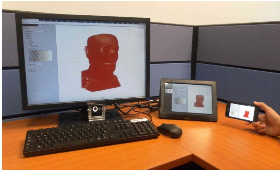
Figure 7-7. WebGL compliant volume rendering of 3D medical dataset by our single-pass GPU ray caster implemented on the stand-alone desktop (left) and two mobile platforms: ACER Iconia A500 tablet (middle) and the Samsung Galaxy SII GT-I9100 mobile phone (right)
