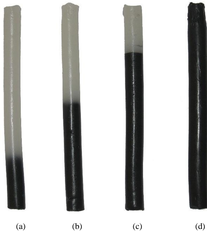
Figure 3-3: Segmented magnet - polymer composites with different doped/undoped proportions: (a) 3cm/10cm, (b) 7cm/6cm, (c) 10cm/3cm and (d) 0cm/13cm
