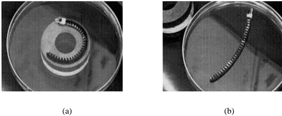
Figure 1-2: Shape distortion of a ferrogel when exposed to a non-uniform magnetic field produced by a permanent magnet: (a) Gel located 15cm from magnet, (b) Magnet placed directly below ferrogel, exhibiting obvious shape change [68].
