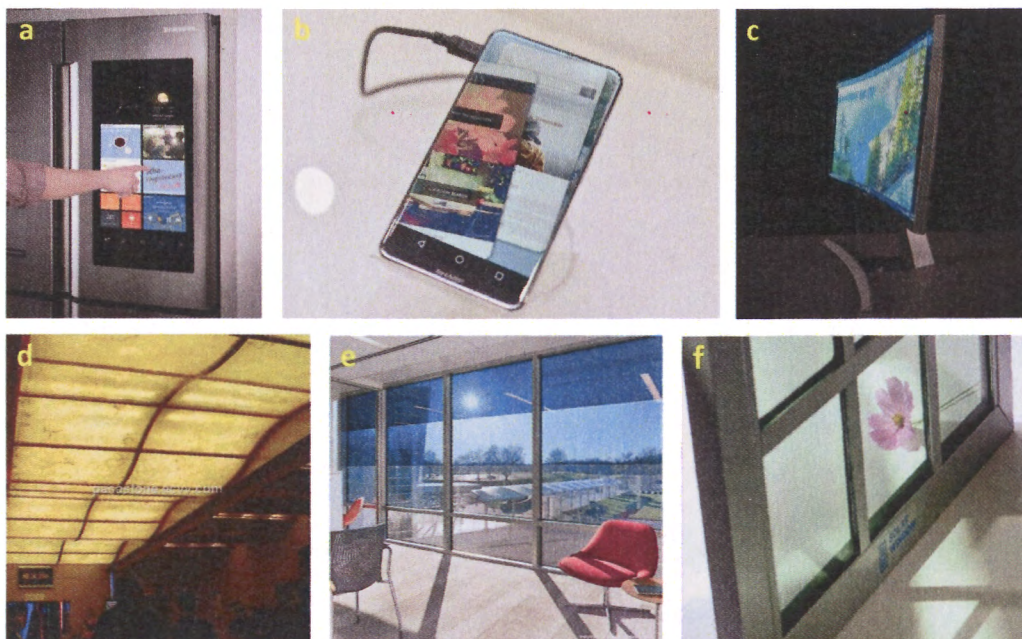
Figure 1.2 Variety of TCL applications: (a), (b) and (c) represent display applications: a refrigerator incorporating a capacitive touch screen [7], a bezel-less smartphone with 2.5D curved display [8] and a monitor with curved display [9], respectively; (d) a luminescent panel [10]; (e) an electrochromic window [11] and (f) a photovoltaic window [12].
