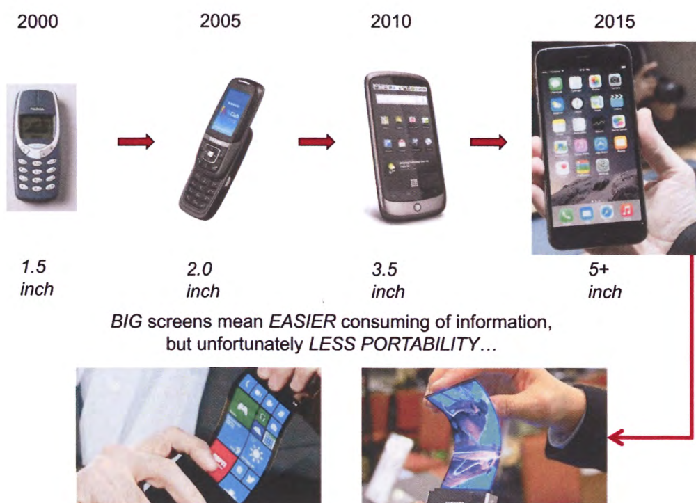
Figure 1.1 Illustration on how the average screen size increased within the last decade based on popular mobile phones [2-6].
