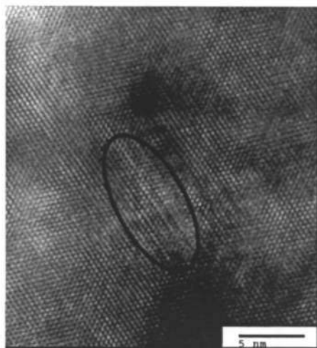
Figure 7.10. HR-TEM image of a dislocation cross-slip at the SiGeC domains area.
