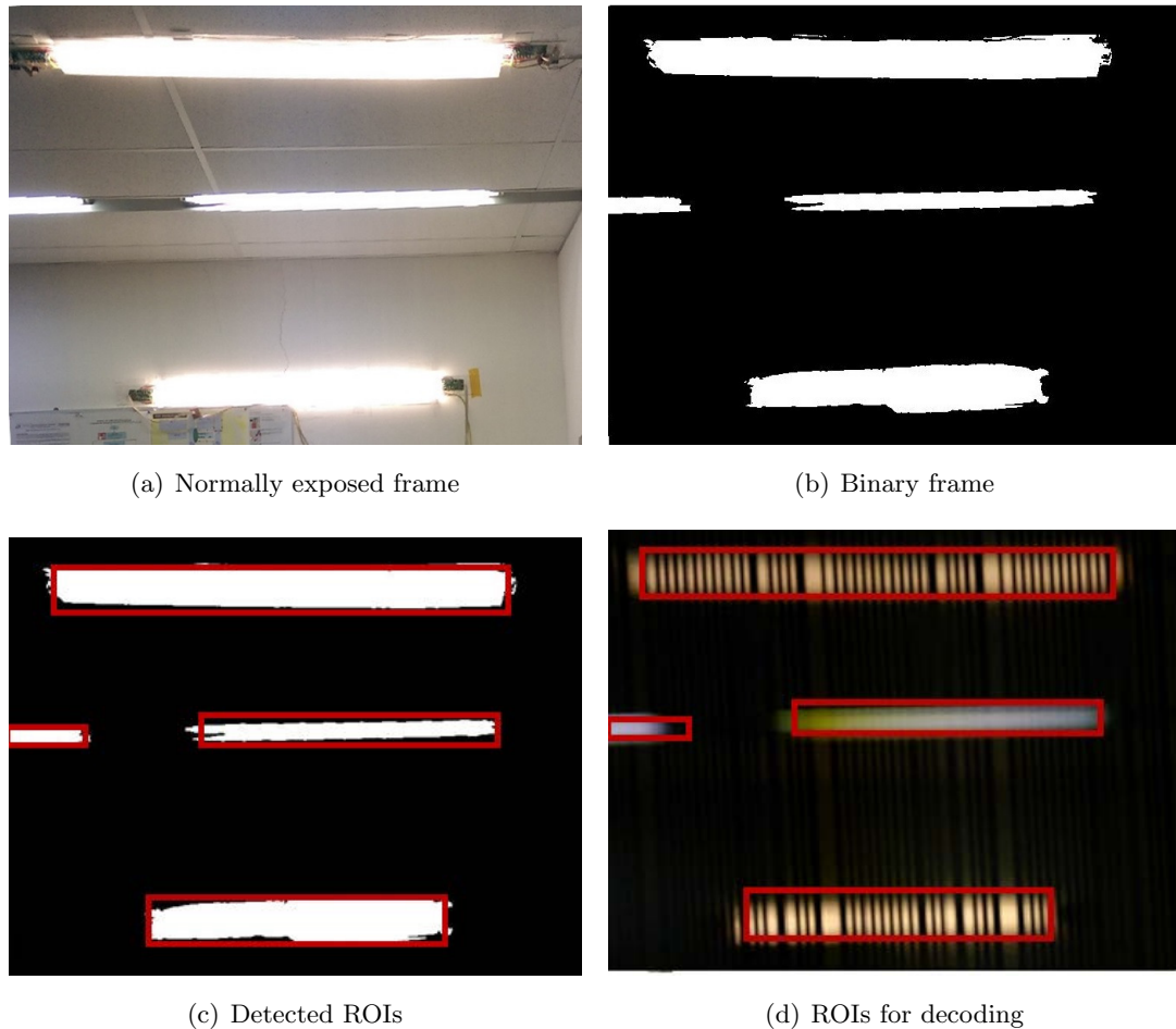
Figure 3.6: Lightweight RoI extraction: for each normally exposed frame (a), we convert it to a binary frame in (b) and detect contours in (c), so that RoIs in a quickly exposed frame (d) can be extracted.
