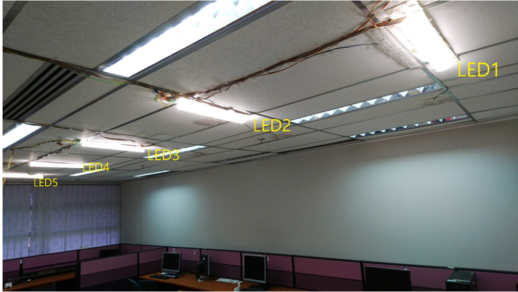
Figure 5.9: RoCLight testbed: five LED luminaires are mounted on the ceiling with an interval of 1.5 m, and the ceiling is 2.5 m above the floor.
