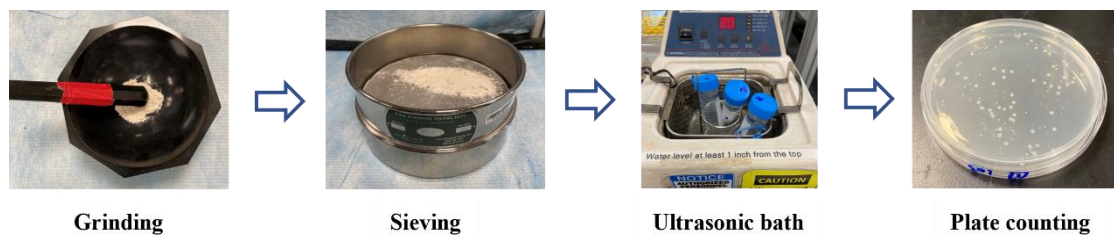
Figure 3.3 The procedure to quantify the bacteria viability in the RMC-B and the PC-B capsules
