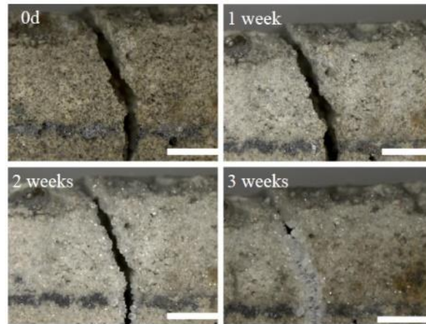
Figure 2.5 Self-healing process induced by melamine-based polymer encapsulated bacteria spores (Wang, Soens et al. 2014)
