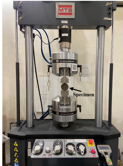
Figure 7.1 Pre-cracking of disc specimen
