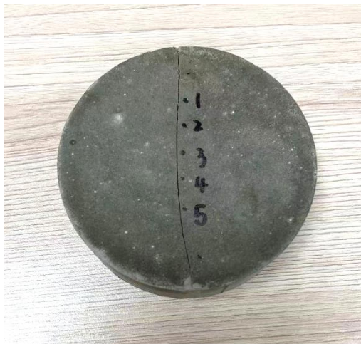
Figure 7.2 A split crack at the center of the specimen after pre-cracking and 5 observation locations along the length of crack on the surface of the disc specimen
