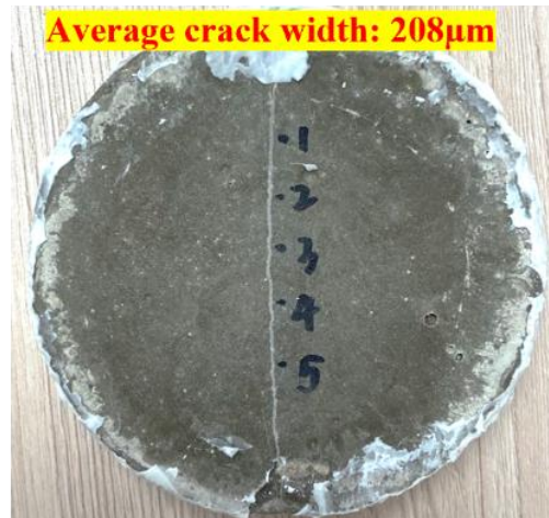
Figure 7.7 A representative fully healed crack in PNC mix
