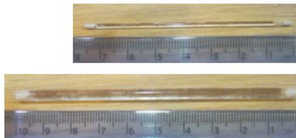
Figure 2.4 Pictures of 1.5 mm and 3.0 mm diameter tubes filled with cyanoacrylate and plugged with wax used for self-healing concrete (Joseph, Jefferson et al. 2010)
