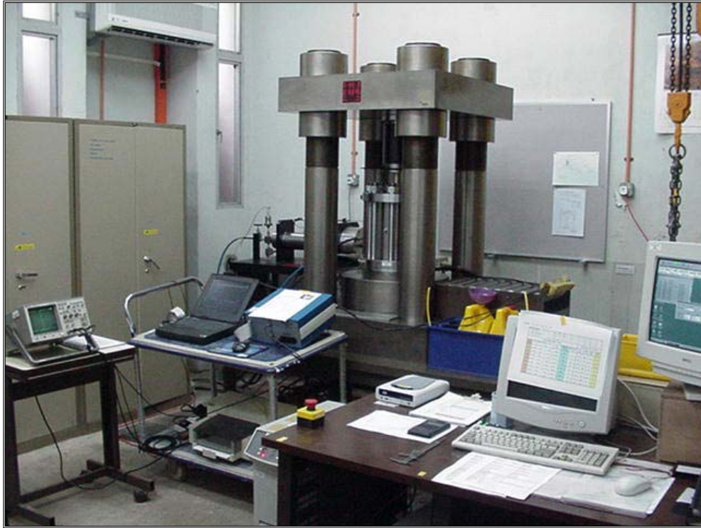
Figure 5.13 STS-1000 machine used for compressive strength testing
