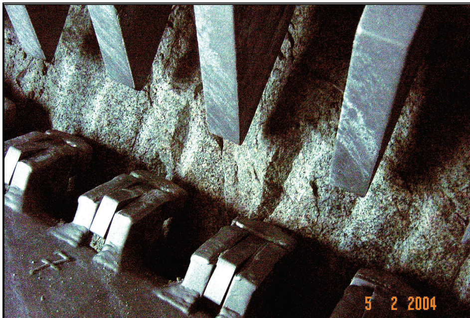
Figure 4.22 Effect of joint orientation on rock chipping formation
