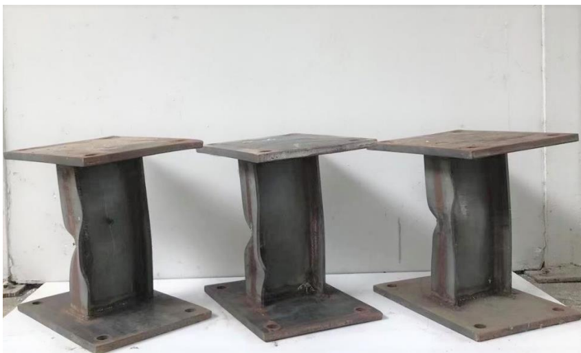
(b) Typical I-150×75×6 specimens (from left to right: D1, D3 and D5)
