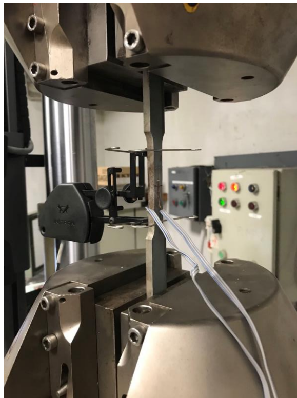
Figure 3.2: Tensile coupon test setup.
