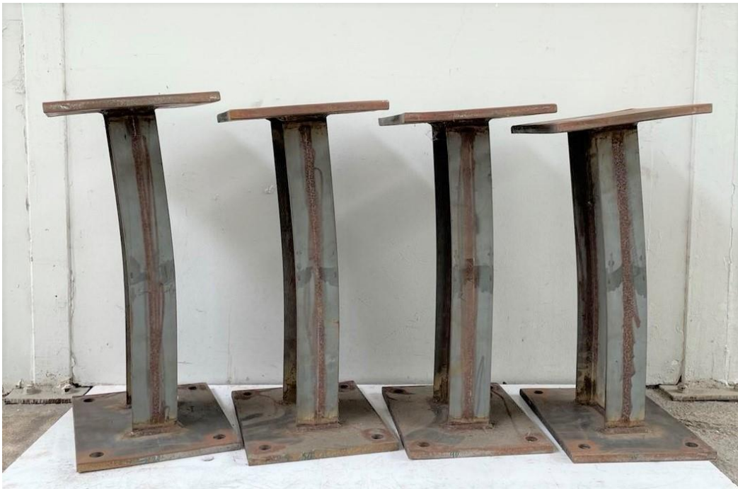
Figure 7.2: Failure modes of I-150×75×6 beam-column specimens.
