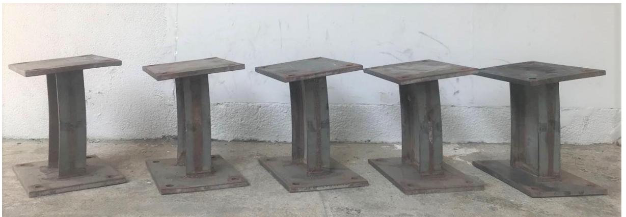
(b) I-150×75×6 specimens (from left to right: B1, B2, B3, B4 and B5).
