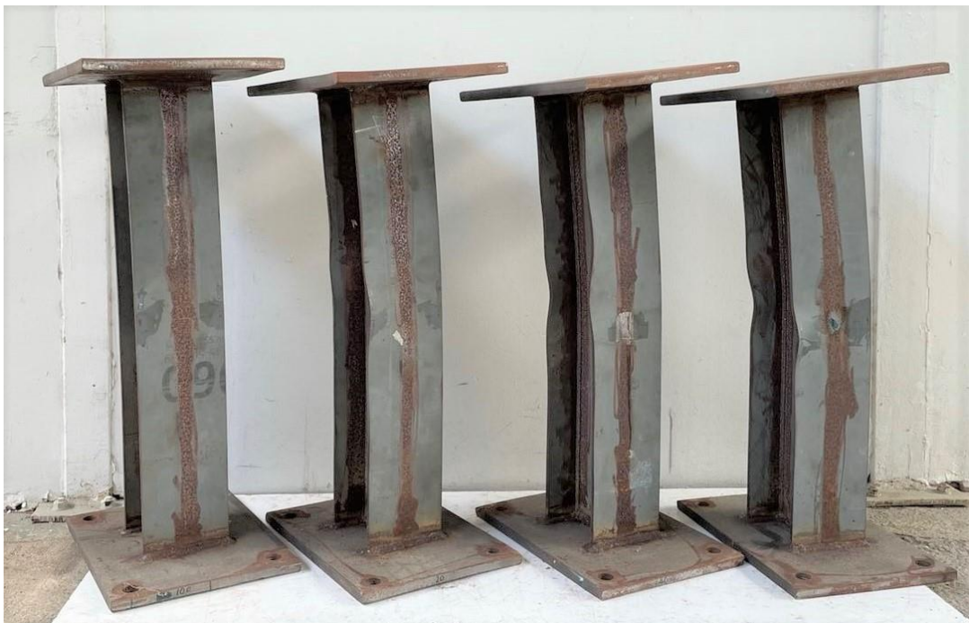
Figure 7.3: Failure modes of I-120×120×6 beam-column specimens.
