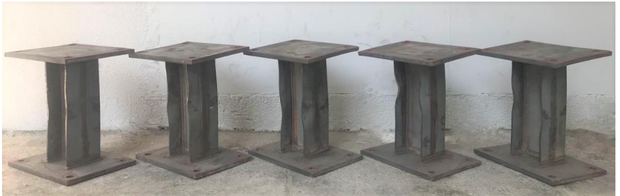
(a) I-120×120×6 specimens (from left to right: A1, A2, A3, A4 and A5).
