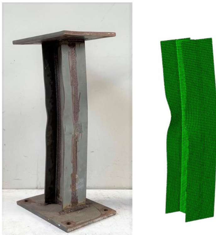
Figure 7.7: Test and numerical failure modes for S960 ultra-high strength steel slender welded I-section beam-column specimen B3.
