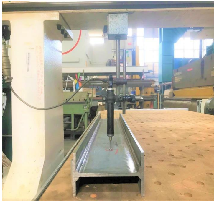
Figure 4.3: Test setup for initial global geometric imperfection measurements.
