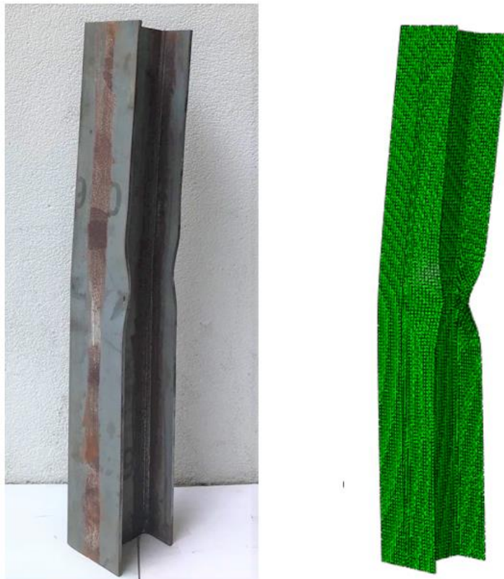
Figure 5.4: Test and numerical failure modes for S960 ultra-high strength steel slender welded I-section column specimen I1-L3.
