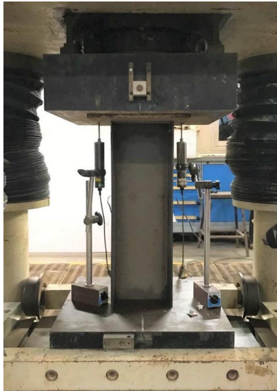
Figure 3.10: Stub column test setup.
