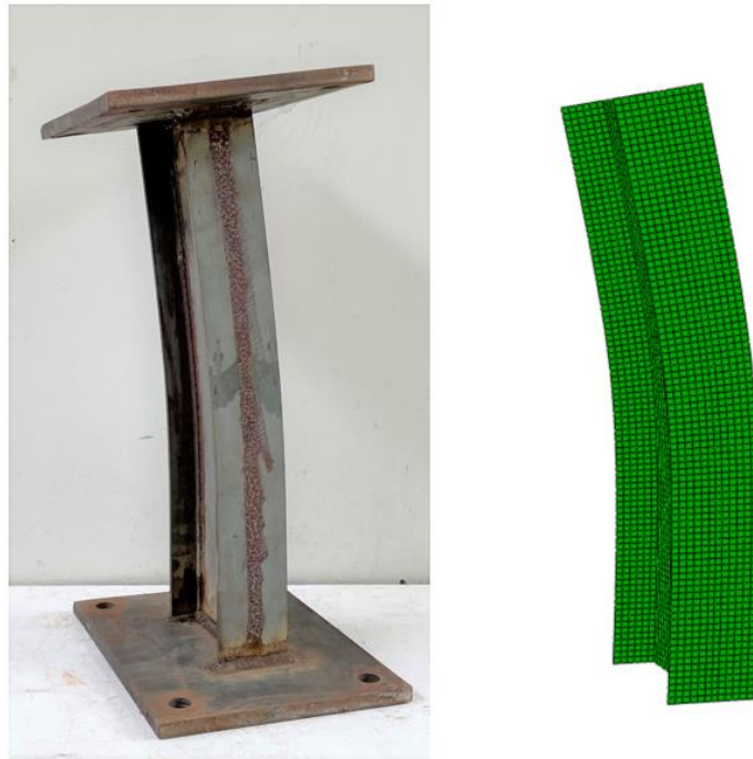
Figure 7.6: Test and numerical failure modes for S960 ultra-high strength steel slender welded I-section beam-column specimen A2.
