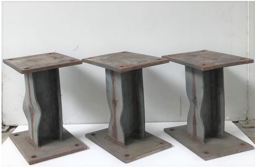
(a) Typical I-120×120×6 specimens (from left to right: C1, C3 and C5)
