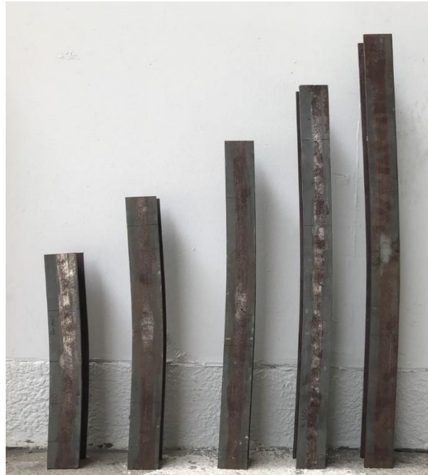
Figure 4.5: Flexural buckling failure modes of typical S960 ultra-high strength steel welded I-section column specimens (from left to right: I1-L1, I1-L2, I1-L3, I1-L4 and I1-L5).
