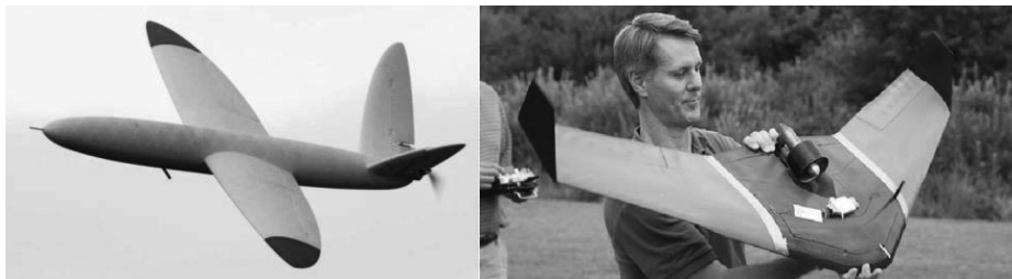
Figure 7. First additively manufactured aircraft and the vehicle from University of Virginia (Chris et al., 2016).
