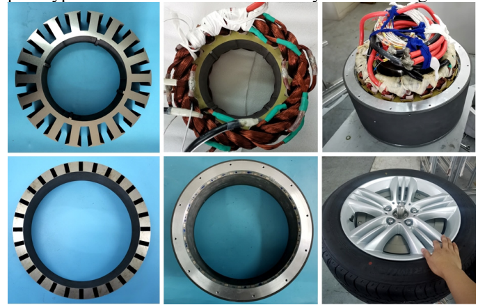
Fig. 6. Mechanical parts prototype MH3 and assembly with 16-inch tire.
