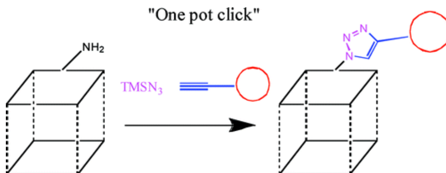
Figure 19. One-pot, two-step functionalization of an amine-containing MOF, DMOF-NH 2 . Reproduced with permission. Adapted with permission from Ref. [199]. Copyright 2010, American Chemical Society.
