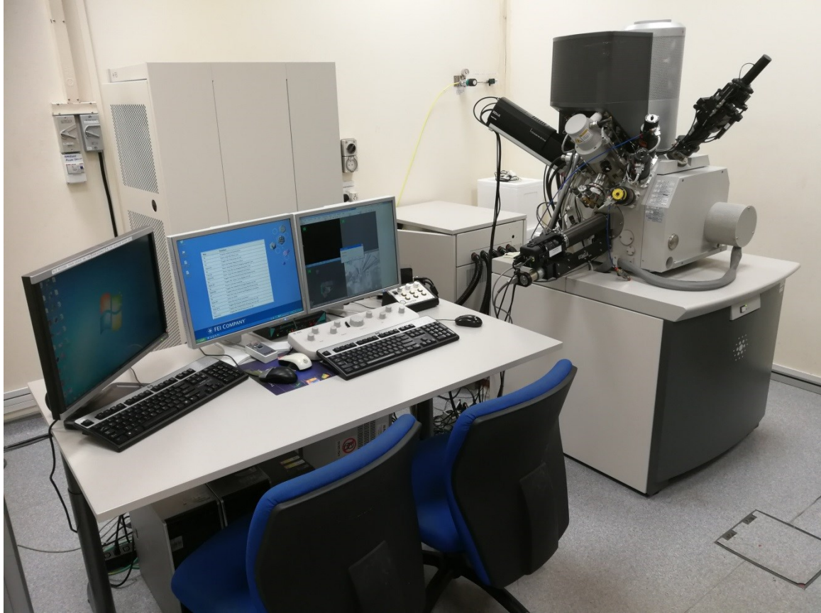
Figure 3.18 Photo of FEI Nova NanoLab 600i FEG-SEM/FIB used in this project
