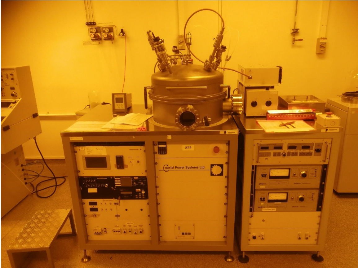
Figure 3.2 Photo of the homemade DC magnetron sputtering system with Sorenson DCS600-1.7E DC power supply unit used in this project
