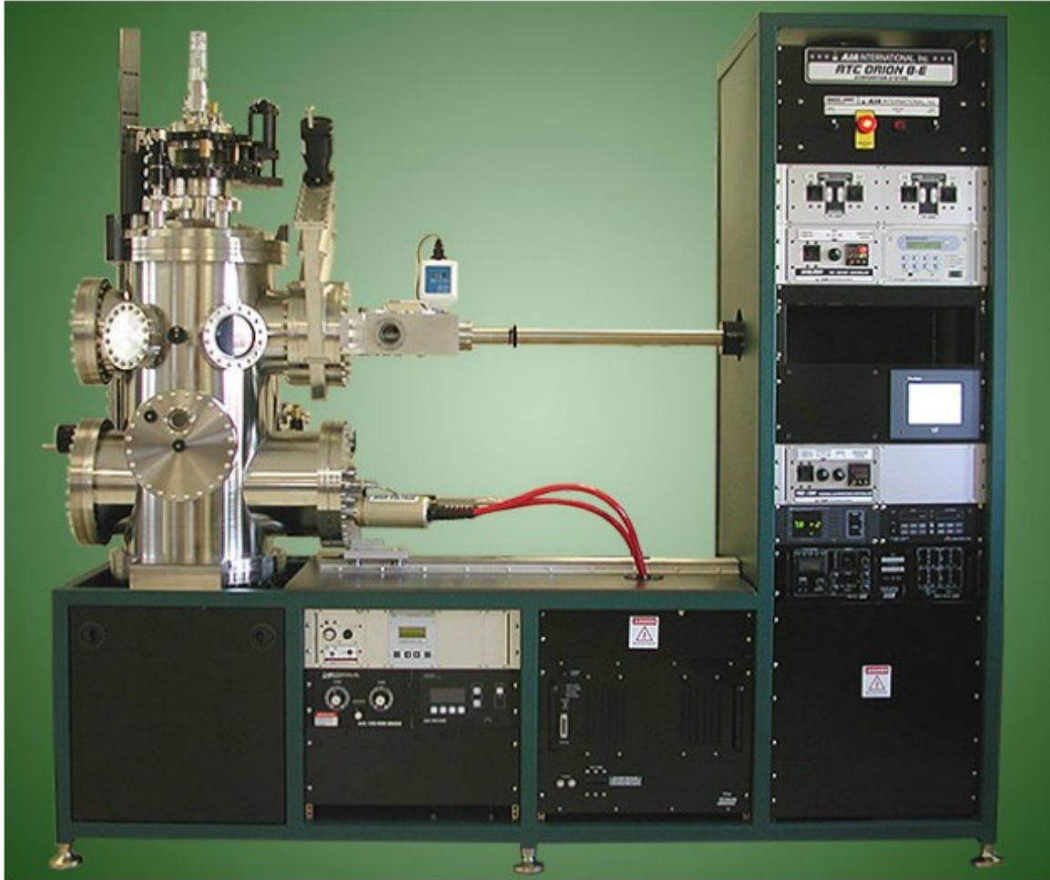
Figure 3.7 Photo of AJA ATC-ORION-8E UHV electron beam evaporation system used in this project
