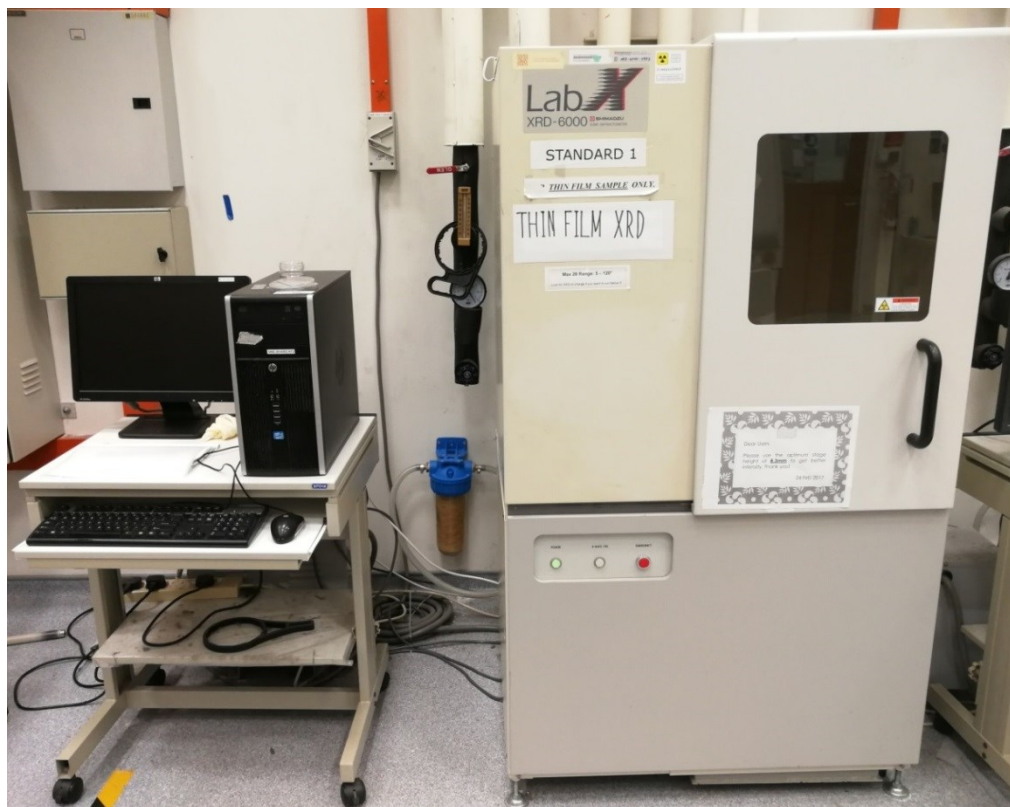
Figure 3.13 Photo of Shimadzu XRD-6000 thin film XRD used in this project
