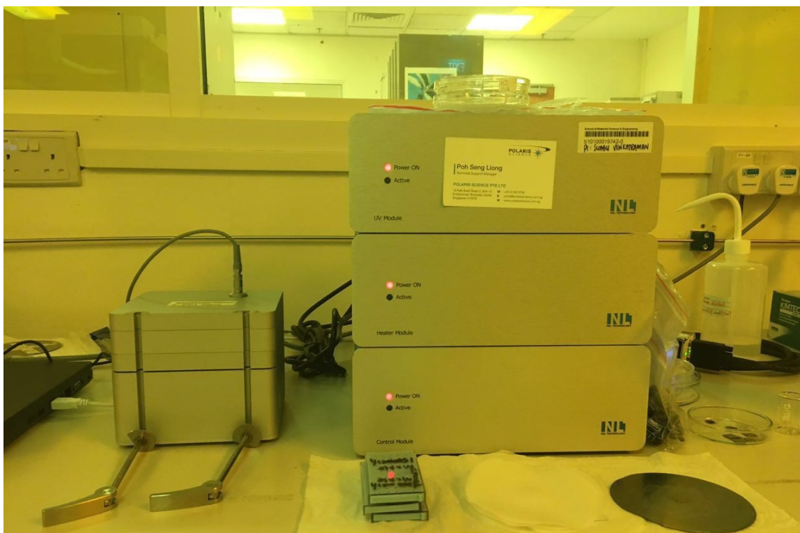
Figure 3.6 Photo of NIL Technology compact nanoimprinter used in this project
