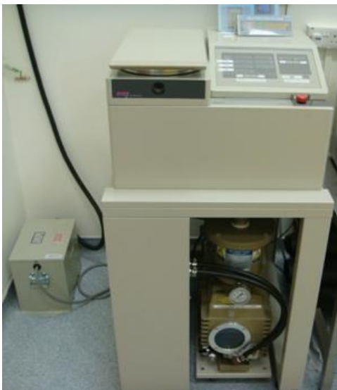
Figure 3.3 Photo of Nippon Scientific ES371 reactive ion etcher used in this project
