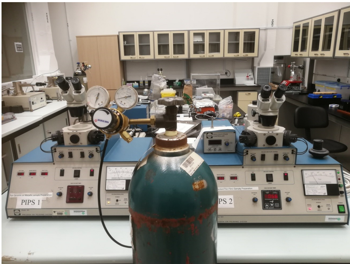
Figure 3.9 Photo of Gatan 691 precision ion polishing system used in this project
