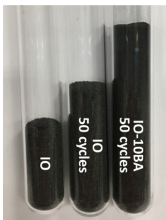
Fig. 8. Volume variation of the OCs after 50 cycles of redox reaction.
