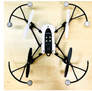
Fig. 18: Motion capture markers on Parrot Mambo
