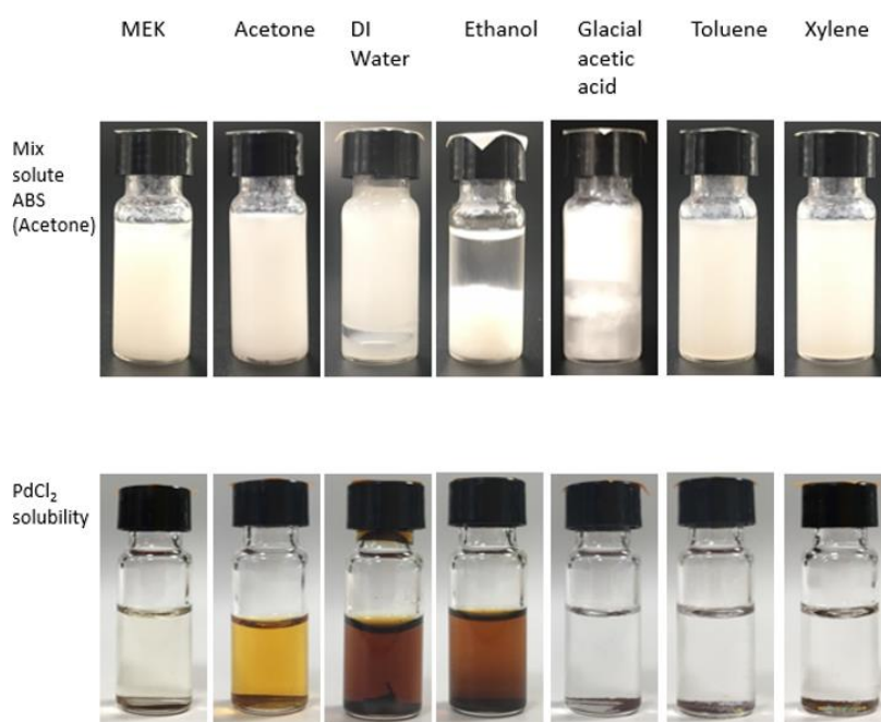
Figure 31 Solvent test by mixing different solvents with solute ABS (acetone) and \text{PdCl}_2 respectively.
