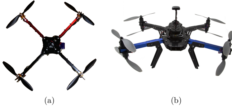
Figure 2.1: A sample quadrotor (a) and its coaxial counterpart (b).
