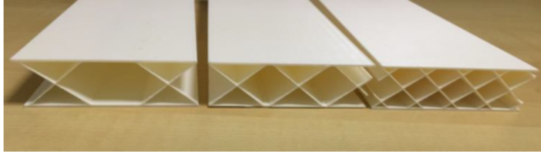
Figure 3.14: Honeycomb structures with different infill ratios: 3%, 5% and 8%.
