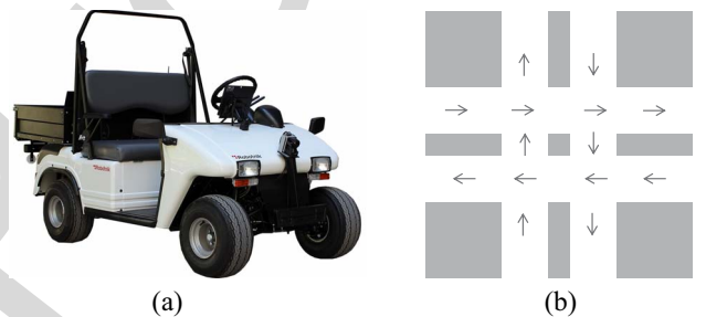
Fig. 13. Example of autonomous car and the schematic diagram of the crossing. (a) RBCAR from Robotnik. (b) Crossing.
