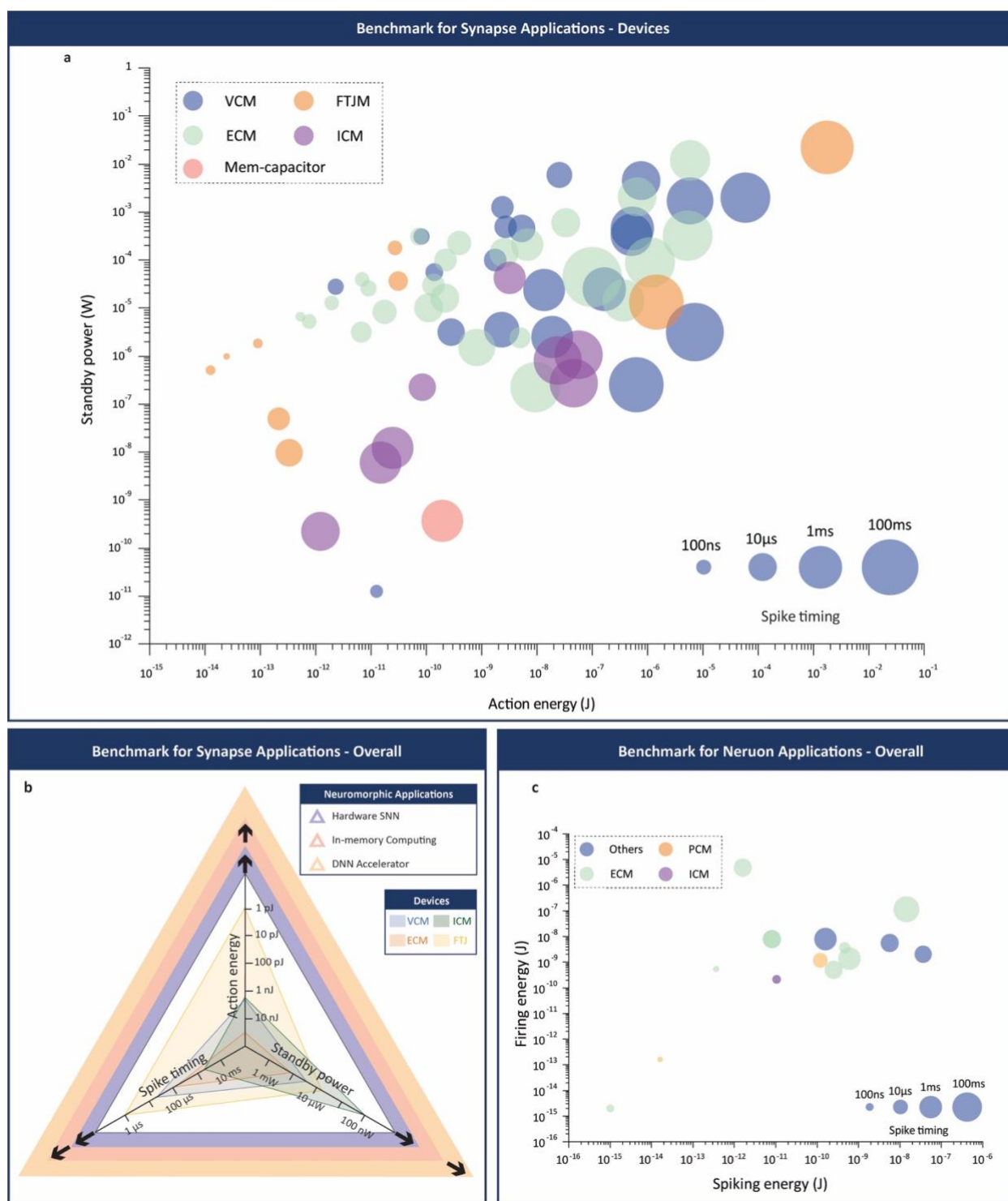
Fig. 11 Universal benchmark for artificial synapse and neuron devices for valence changing memristive device (VCM), electrochemically metallization memristive device (ECM), interface-controlled memristive device (ICM), ferroelectric tunnelling junction device (FTJM), and mem-capacitor. a , Benchmark for synapse applications, where standby power is a function of action energy and the diameter of the bubble indicates the spike timing of the device. b , Overall performance comparison of artificial synaptic devices based on the median of each device group in the benchmark. The outer frame suggests possible neuromorphic application direction. c , Benchmark for neuron applications, where firing energy is a function of spiking energy. Credits: VCM data are extracted from ref. 94, 95, 97, 98, 100, 102-108, 114-116, 124-126, 213-220 , ECM data are extracted from ref. 69, 122, 123, 220-228 , ICM data are extracted from ref. 88, 149-154, 229 , and FTJM data are extracted from ref. 70, 198, 200, 204-207, 230, 231 , mem-capacitor data is extracted from ref. 210 , artificial neuron data are extracted from ref. 142, 173, 232-243 .
