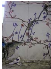
(e) Crushing of the two columns at the bottom edges at DF = \pm 6
