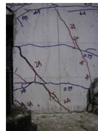
(e) Crushing of the two columns at the bottom edges at DF = \pm 6
