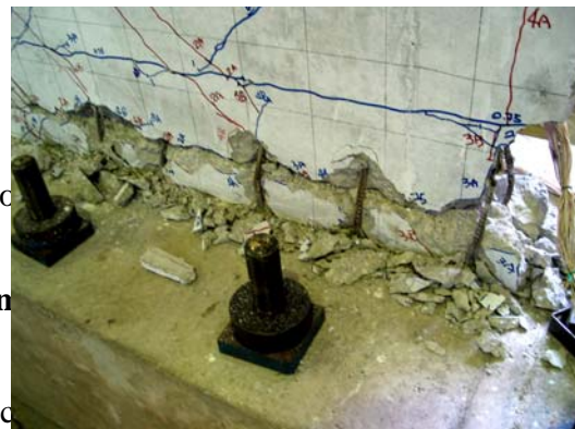
(c) Bottom sliding face formed at DF = \pm 3
