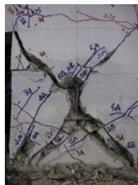
(f) Damage of the four bottom columns at DF = \pm 7
