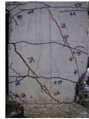
(e) Crushing of the two columns at the bottom edges at DF = \pm 6
