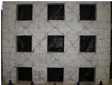
(c) Diagonal cracks at DF = \pm 4
