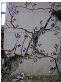
(e) Crushing of the two columns at the bottom edges at DF = \pm 6
