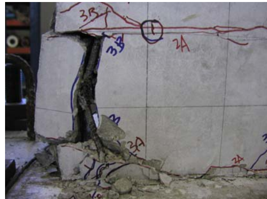
(b) Buckling of reinforcing bars at DF = \pm 4
