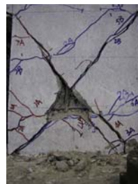
(f) Damage of the four bottom columns at DF = \pm 7
