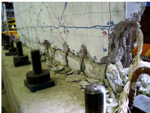
(c) Bottom sliding face formed at DF = \pm 3
