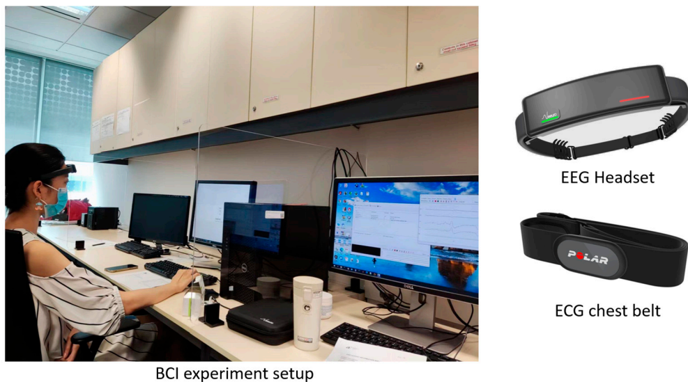
Figure 3. Example of the experimental setup. The right-side screen enabled the operator to monitor the EEG/ECG signals and data acquisition process. The left-side screen was for displaying visual cues to the participant for the cognitive tasks. Each participant wore an EEG headband on their forehead, and an ECG chest belt.
