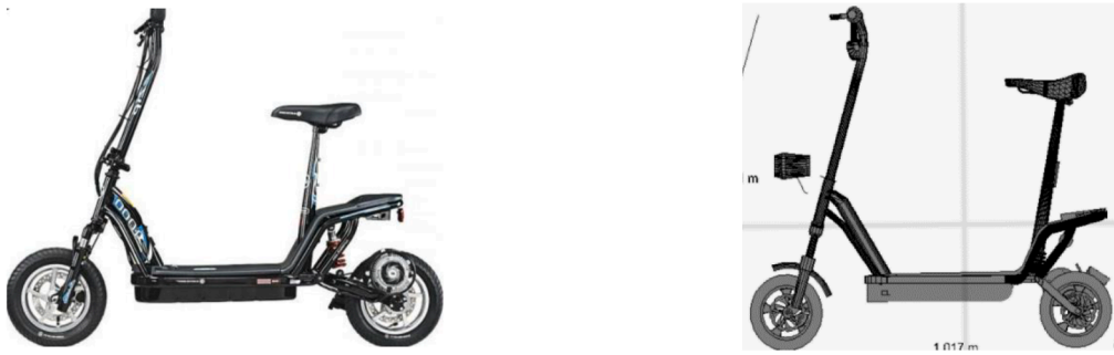
Fig. 2. E-scooter model (left- actual e-scooter mode, right- Virtual Crash model).
