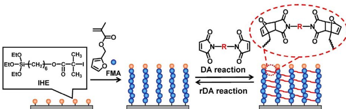
Scheme 2. Schematic Illustration of Synthesis of PFMA Brush and Reversible Crosslinking and Decrosslinking of PFMA Brush via DA and rDA reactions.
