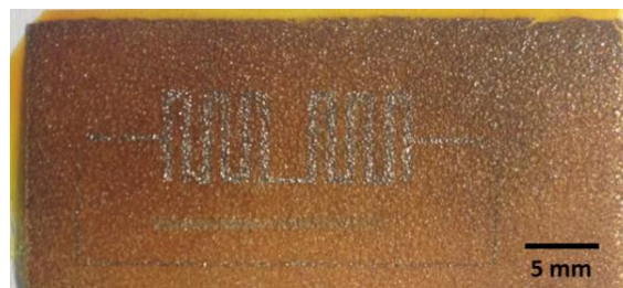
Figure 6-10. Printed electronic resistor on 3D-BN/PI film
