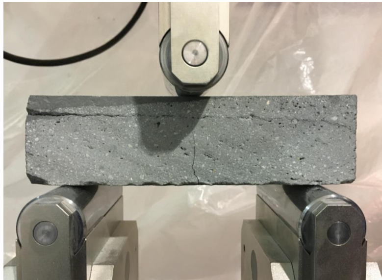
Figure 6.20 The failure status of geopolymer mortar
