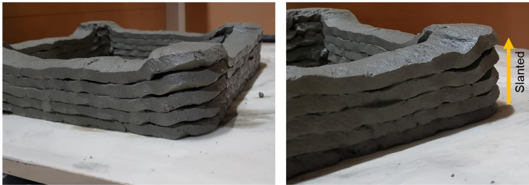
Figure 6.6 Example of layer stacking at the corner due to sharp turn curvature and small layer width
