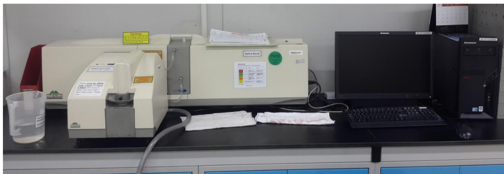
Figure 3.17 Malvern Mastersizer 2000 instrument used for PSD analysis of powder samples and flocculated colloidal
