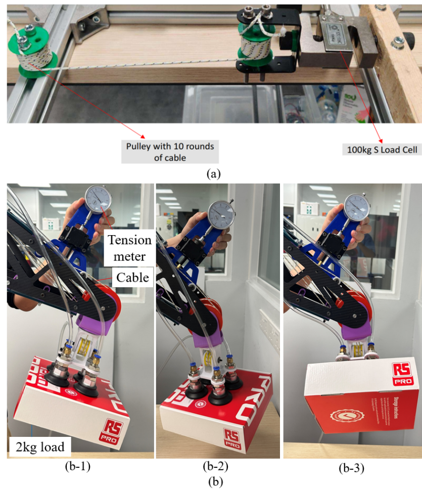
Figure 11. Setting up experiments for testing the cable loosening in static payload of 100 kg (a) and dynamic payload of 2 kg (b) with (b-1), (b-2), and (b-3), respectively, for rotating around z_3, z_4, z_5 .
