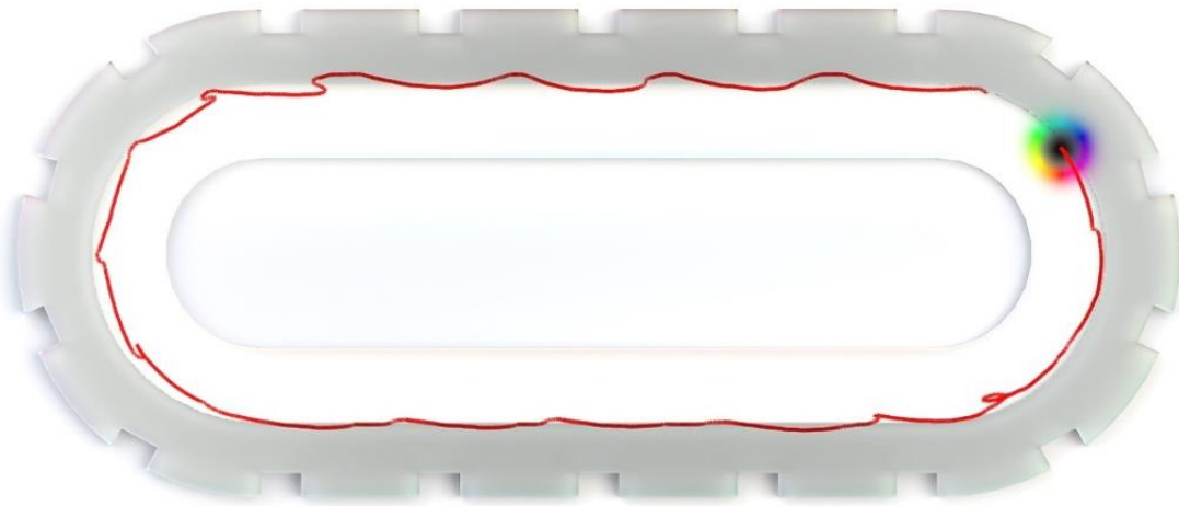
Figure 4-17 Image of a recirculating skyrmion ratchet where the red line represents the skyrmion trajectory. To shift the skyrmion by a step, a voltage pulse of 0.8 ns was applied followed by a 1 ns interval for the skyrmion to relax into the potential well.
