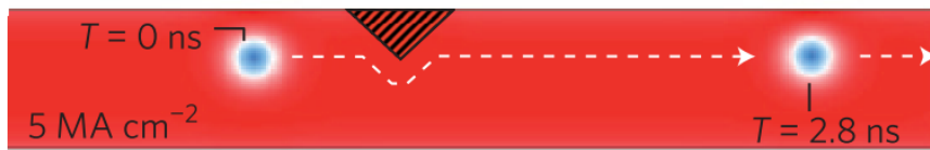
Figure 1-10 Trajectory (white dotted line) of a skyrmion moving past a barrier. The skyrmion deflects lightly to avoid the pinning site (shaded triangle). 54
