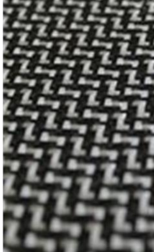
Figure 2.16. Novel woven fabric developed by DSM; an intralayer of carbon and ultrahigh molecular weight polyethylene fibre.
