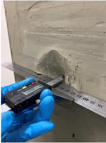
Figure 3.4. A vernier calliper was used to measure the back face signature which corresponds to the deepest point made on the Roma Plastilina clay backing post-impact.
