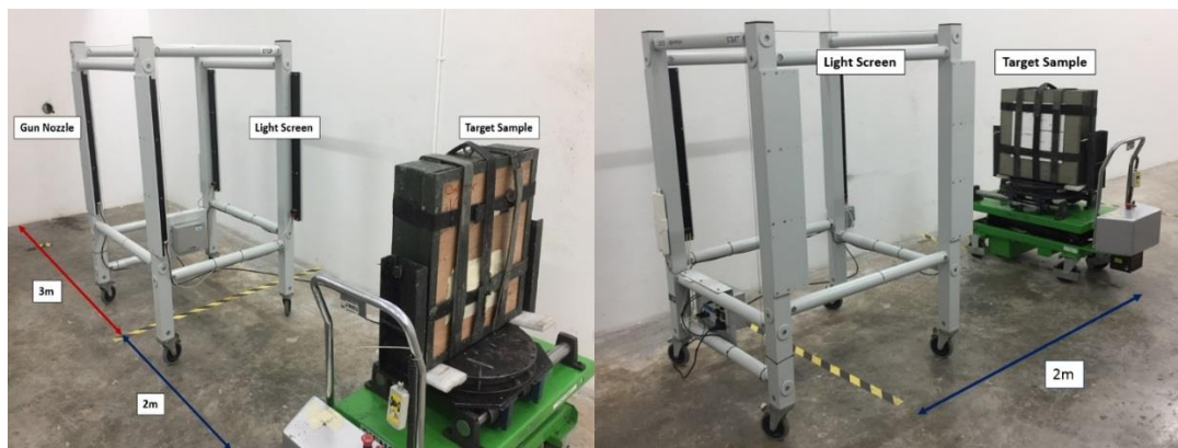
Figure 3.3. Ballistic test set up; Light screen for projectile velocity determination was placed 3 metres away from the gun nozzle and the target sample was placed 5 metres from the gun nozzle.
