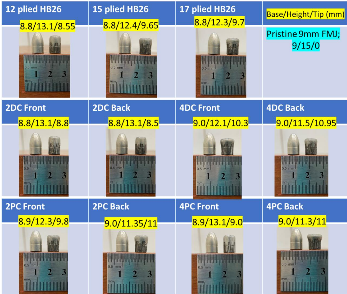
Figure 6.4. Comparison of the base, height and tip changes post-impact of a 9mm FMJ projectile on the various composite panels.
