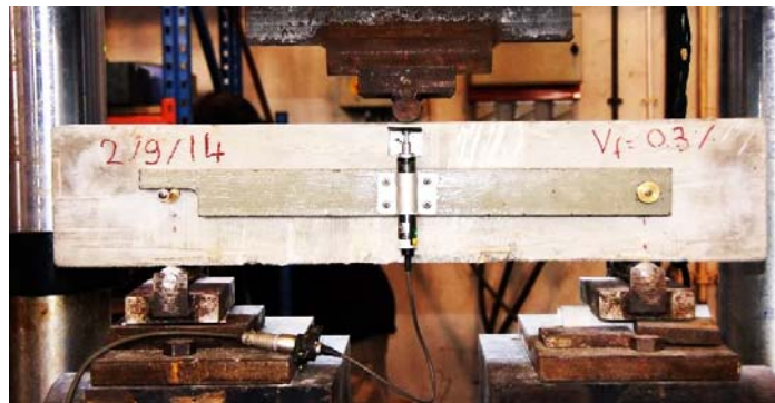
Fig.4. 7 – Photograph from the notched beam test according to EN 14651:2007
