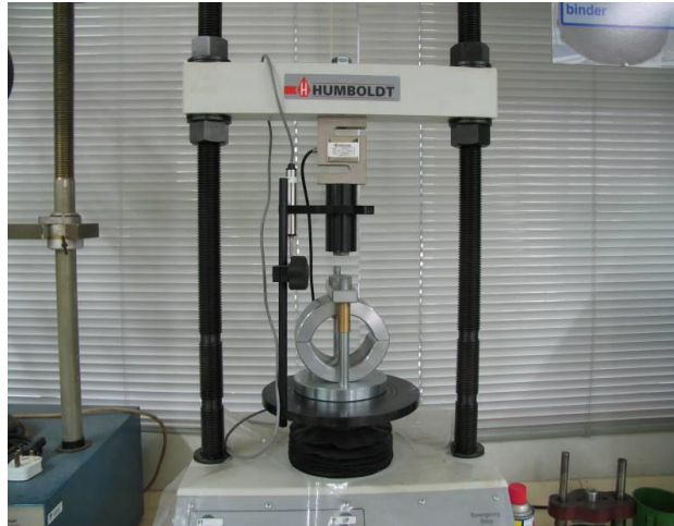
Figure 3.4 Apparatus for Marshall test
