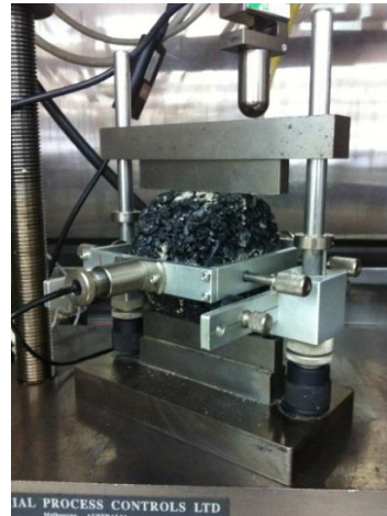
Figure 3.5 Apparatus for ITSM test
