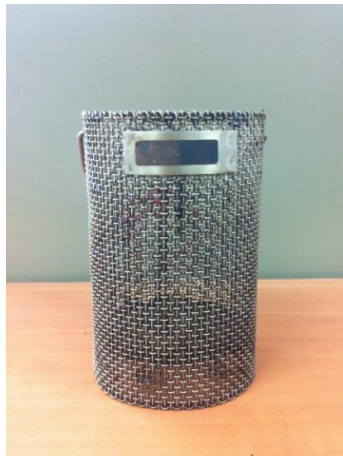
Figure 3.2 Wire basket used in draindown test
