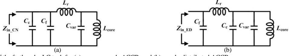
Fig. 6. Schematic of the fourth-order LC tank for (a) common-node ACCPs and (b) evenly-distributed ACCPs.
