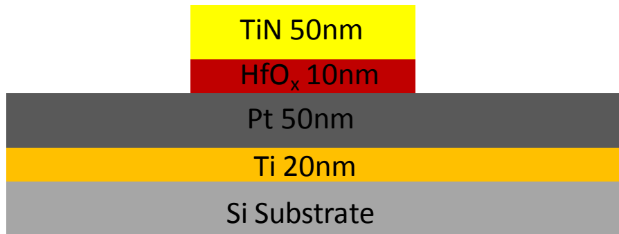
Figure 5.1 Schematic of the memory cell (DUT) used in current conduction mechanism investigation via both DC and LFN analysis. TiN and Pt are used as top and bottom electrode respectively and 10nm of HfO x is used as resistive switching layer.
