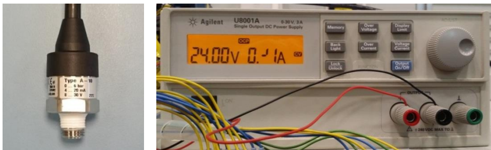
Figure 5-20: (a) WIKA pressure transmitter and (b) Agilent DC power supply unit
