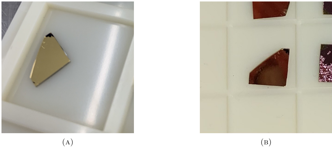
FIGURE 3.4: A Silicon substrate coated with gold and HSQ before annealing. B Silicon substrate coated with gold and HSQ after annealing, showing significant degradation of gold layer.
