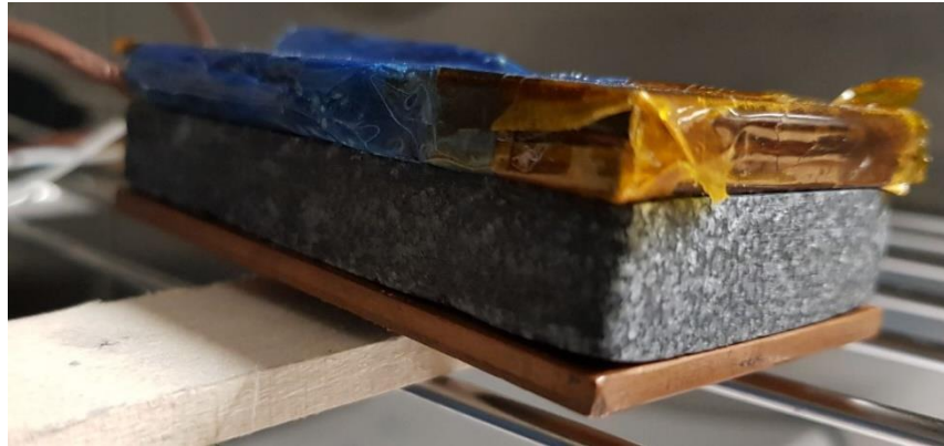
Figure 3.9 Actual set-up of the Lee's disc method with a sample of 3DCPCM.
