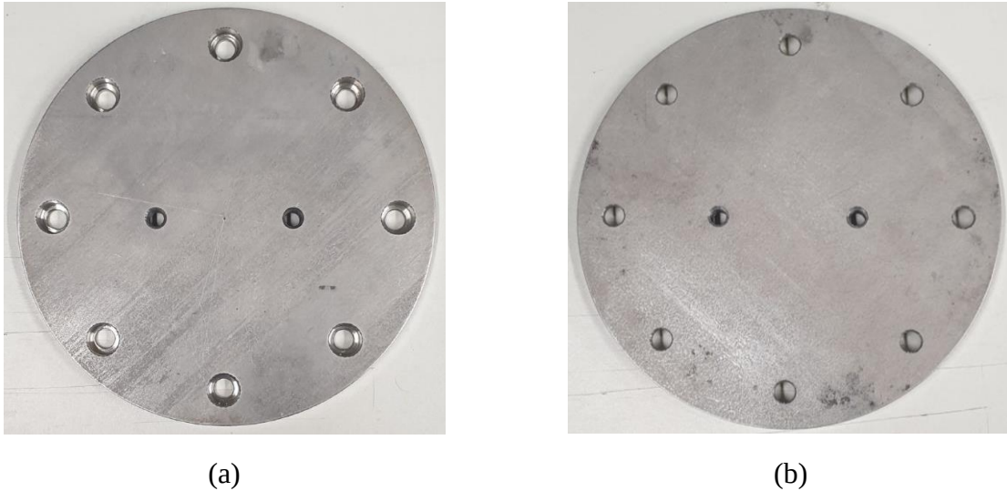
Figure 7.3 Stainless steel mounting plate with eight M8 attachment points along a 150 mm circumference for attachment to the shaker vibration plate and two M8 threaded inserts for mounting of the PCM fixture. (a) top view (b) bottom view, in contact with the shaker vibration plate.
