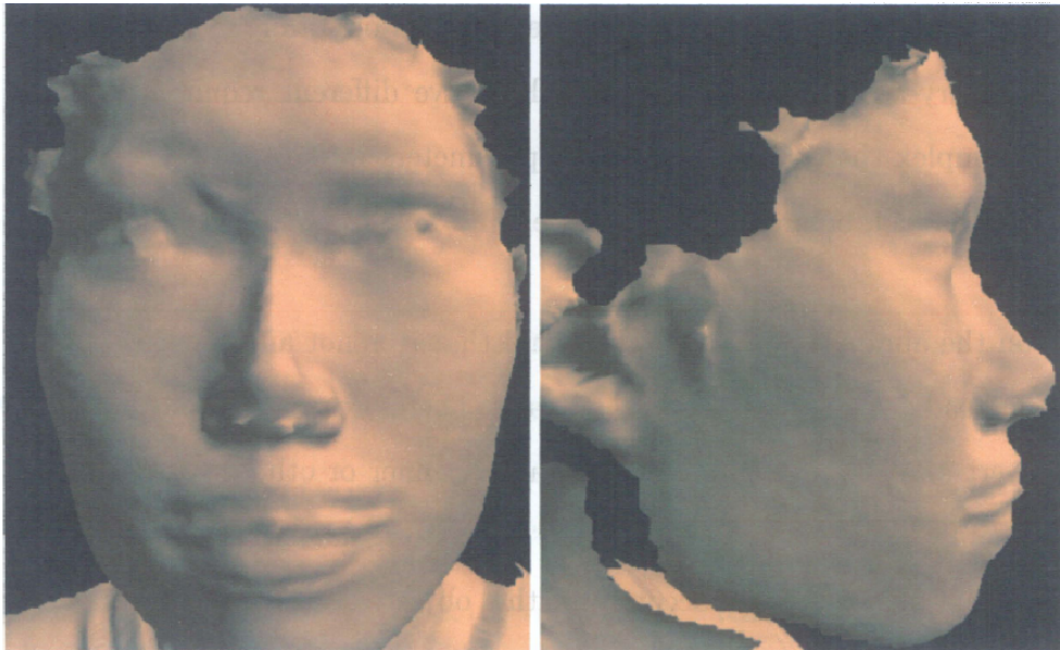
Figure 4.1: Range scan data from Minolta Vivid 700 Laser Scanner
