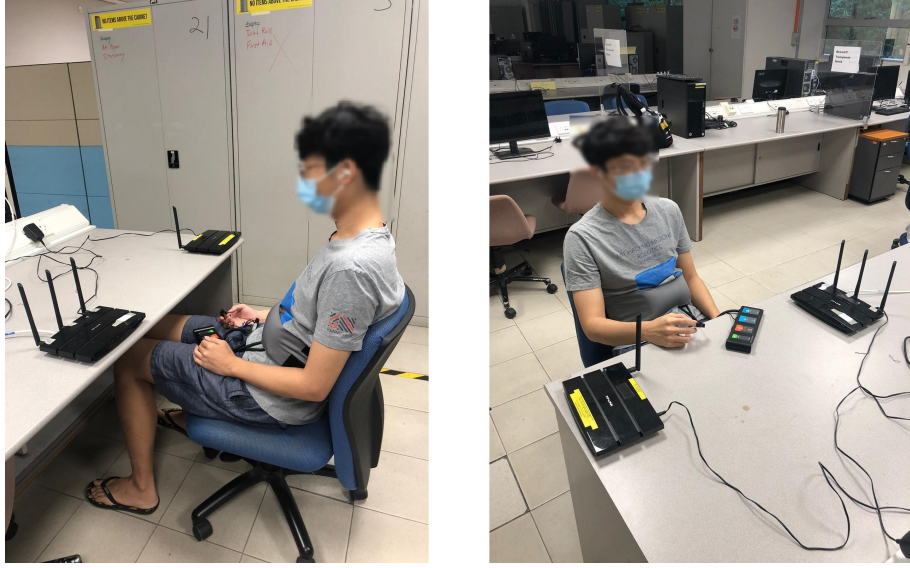
Figure 7.6: Experimental setup with the WiFi transmitter and receiver positioned in aligned (left) or parallel (right) with respect to each other.
