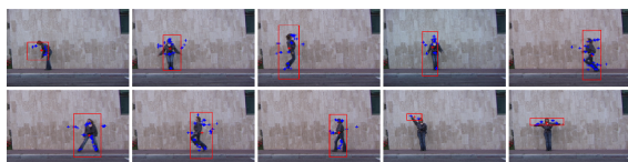
Figure 3: The localization of ten action classes in the Weizmann dataset. Computed centers of actions is marked with a red cross-hair. The local action windows are marked by red rectangles.
