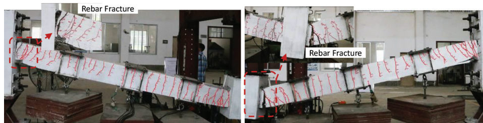
Fig. 10—Failure mode of PC specimen PCSH-0.6.
