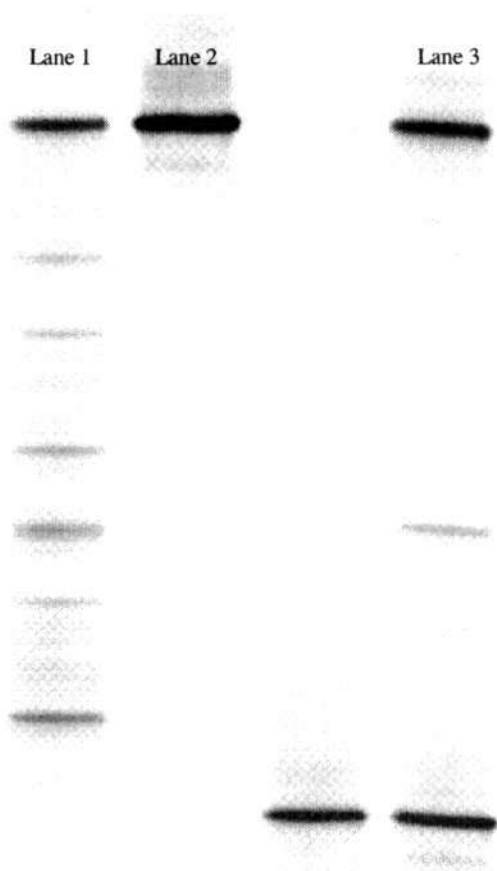
Figure 6.1 Denaturing gradient gel electrophoresis (DGGE) fingerprints of PCR-amplified 16S rRNA fragments from aerobic granules cultivated in previous experiment as described in Chapter Four. Lane 1: phenol-degrading granule seeded by acetate-fed granule; Lane 2: strain S15; and Lane 3: acetate-fed granule as bioseed for the cultivation of phenol-degrading granule
