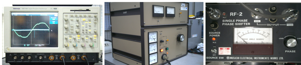
Figure 3-6 Testing equipments: (L) Panel of Tektronix TDS 7104 Digital Phosphor Oscilloscope; (M) HV series control unit; (R) Phase shifter panel
