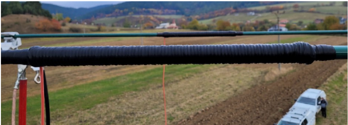
(b) An SLI sensor with semi-conductive insulation.
