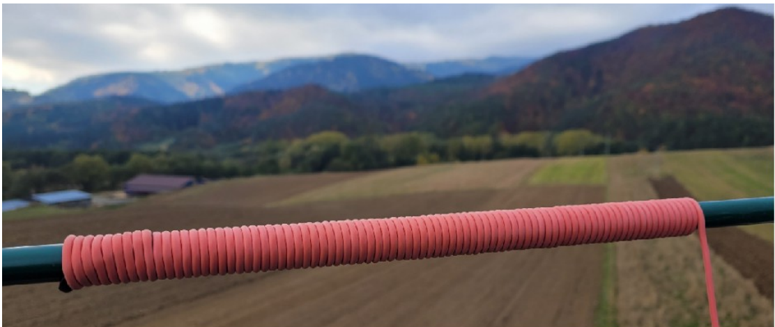
(a) An SLI sensor (red) during installation.
