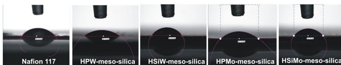
Figure 7.3 Water contact angle on the surface of Nafion 117, HPW-meso-silica, HSiW-meso-silica, HPMo-meso-silica and HSiMo-meso-silica membrane
