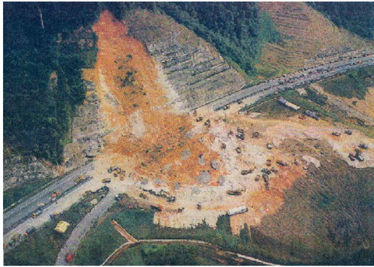
Figure 7.4 A deep rotational slide at Langkawi, Malaysia (from Huat et al., 2006)
