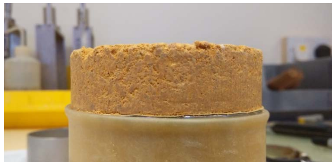
Figure 3.13 Soil specimen ( w = 16.2\% ) after the cyclic and monotonic shearing
