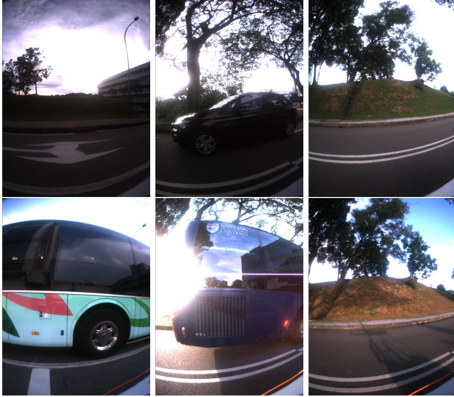
Figure 5.7: The database and query images of the three circles marked in Fig. 5.6b. The top images show the views obtained from the database for the estimated vehicle location. The bottom images show the views of the query image of the current position. Only one view of the six cameras is shown here.
