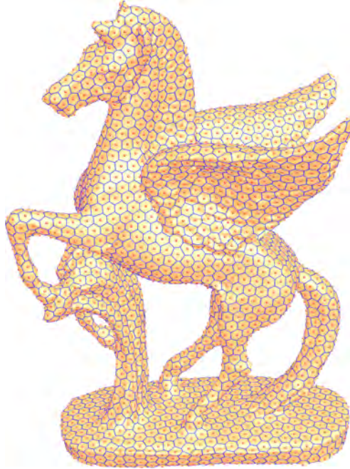
Figure 5.1: Our intrinsic method can compute a high-quality centroidal Voronoi tessellation on model with complicated geometry and topology. The CVT on the Pegasus model was created by 3000 sites.
