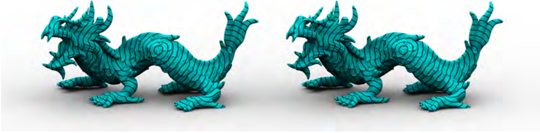
Exact polyhedral distance: ICH 127s; MMP 144s Our result: 1.96s, max err. 0.11%, rms err. 0.05%, mean err. 0.04%
